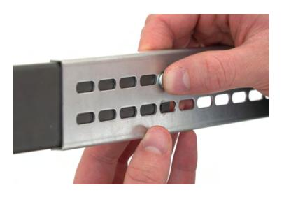
Pinch the Rear Extension Bracket and rail outer member together. Feed 1x M-4 Pan Head screw through the obround hole and the hole in the outer member.
