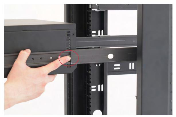
Insert the the inner slides into the extended outer members. You will need to depress the security latches on the outer member as you do so. Push the chassis until you hear the security latches engage, pictured below.
