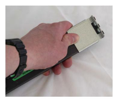
Hold 1x Front Support Bracket against the front prongs of the rail slide outer member, as shown on the left. Make sure the bracket is flush against both the outer member and the front prongs.
