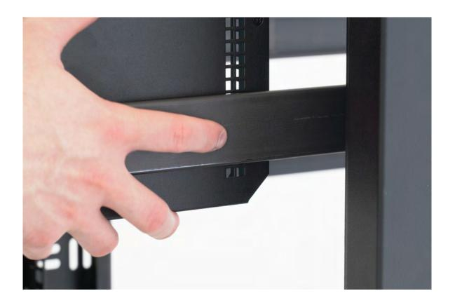
Once the inner slides are successfully centered and slide into the middle members, you will need to press down the security latches to finish sliding the chassis into your rack cabinet. The second set of security latches will disengage automatically as you slide the chassis all the way in.
